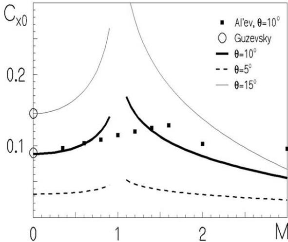
Fig 2. Calculations of the  $c_{x0}$  values for different conical cavitators. Slender body theory (eqs. (13) and (14), [22, 25]) are represented by lines, non-linear numerical methods [27, 28] – by markers
