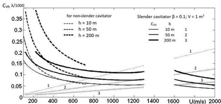
Fig 4. Drag coefficients  $C_{Vh}$  ( $\gamma = 1$ ) and the cavator+cavity aspect ratio at different values of the depth  $h = 10; 50; 200$  m (the thickness of the lines is increasing with the depth).  $C_{Vh}$  for disc and non-slender conical cavitators, eq. (3), (15) – dashed lines; for the slender conical cavitator, eqs. (11) – (15),  $\beta = 0.1$ ;  $V = 1\text{ m}^3$  - solid lines. Values  $\lambda/1000$  for the slender conical cavitator, eq. (11),  $\beta = 0.1$  -- dotted lines
