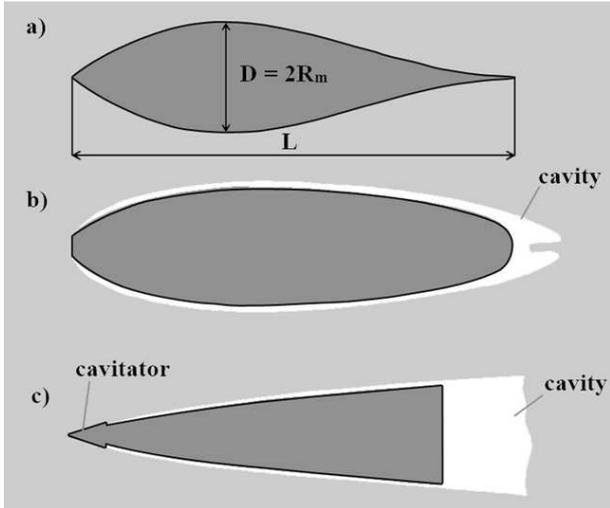
Fig. 1. Different axisymmetric underwater flow patterns:
